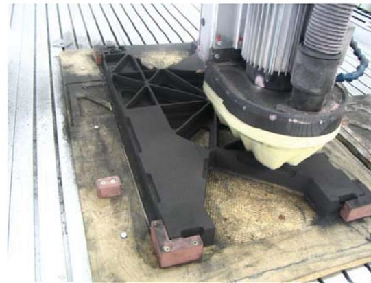
Fig. 9. HSOB plate-form greenbody during milling
