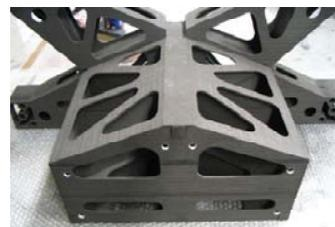
Fig. 13. View of HSOB greenbody once assembled
