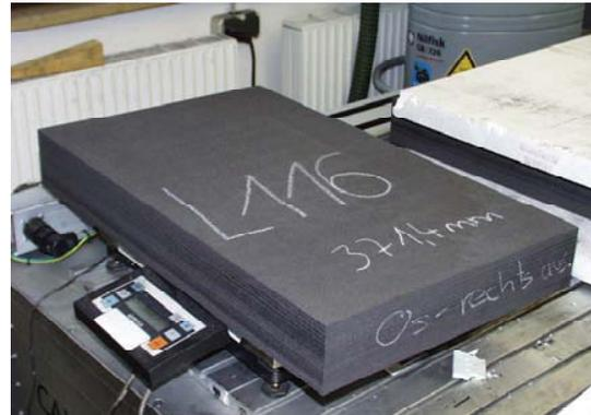
Fig. 8. View of a C/C block after cut
