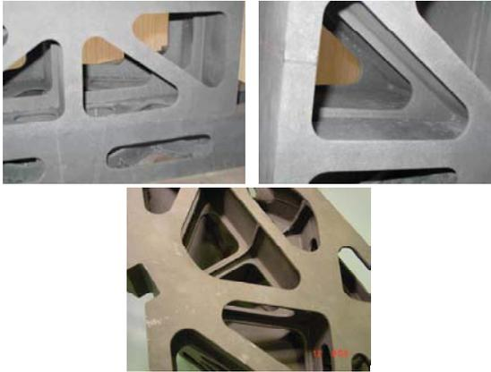
Fig. 10. HSOB inner cells due to ribs & skins
