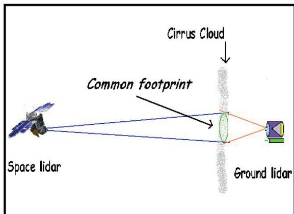
Figure 3: Schematic diagram of the different beam divergences between the space and ground based lidars. The so called common footprint is shown.
