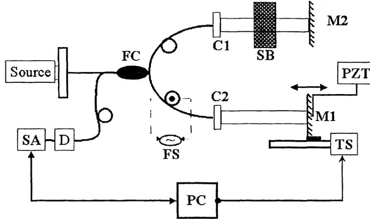
Figure 2: Experimental setup for ballistic waves attenuation through a scattering background. FC fiber coupler; C1, C2 collimators; SB scattering background; M1, M2 mirrors; PZT piezoelectric transducer; TS translation stage; FS fiber stretcher; D detector; SA spectrum analyzer; PC personal computer.
