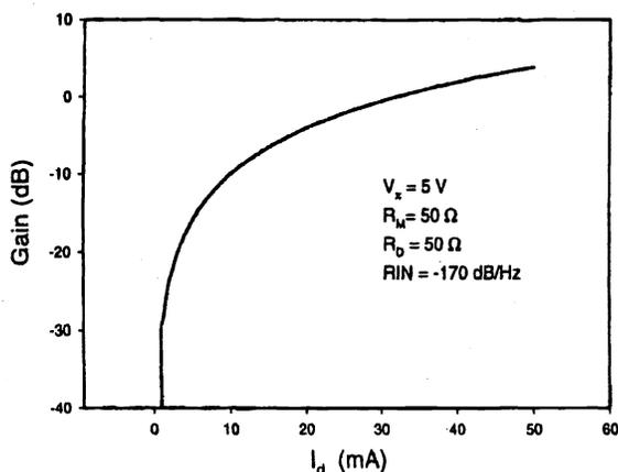
Figure 3: Link Gains vs. Photodetector Current
