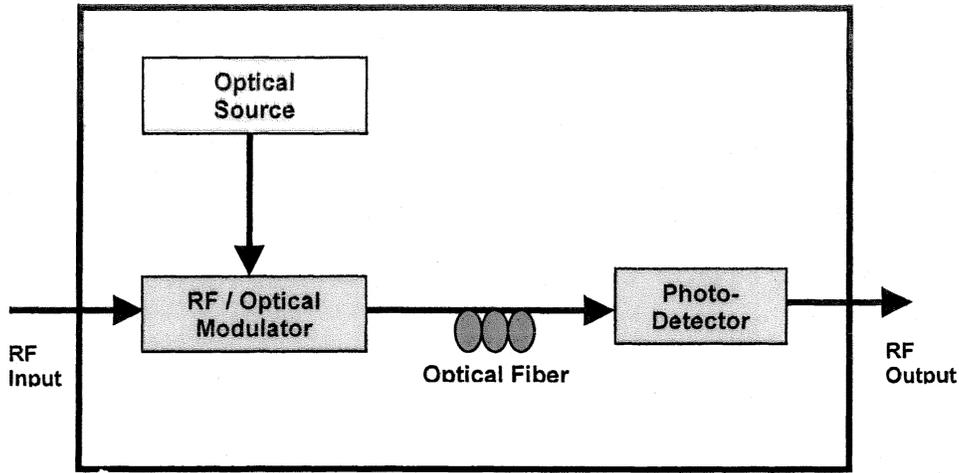
Figure 1: RF Fiberoptic Link
