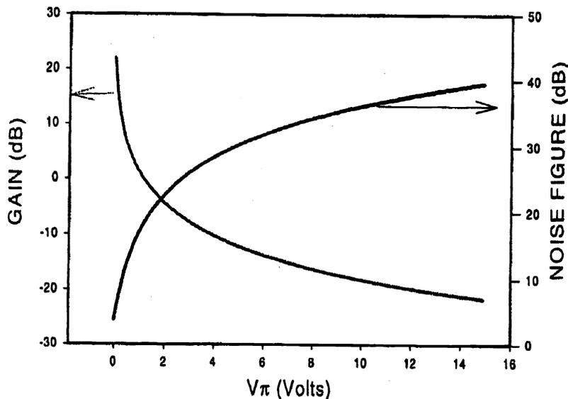
Figure 2: Link Gain and Noise Figure vs.  $V_\pi$
