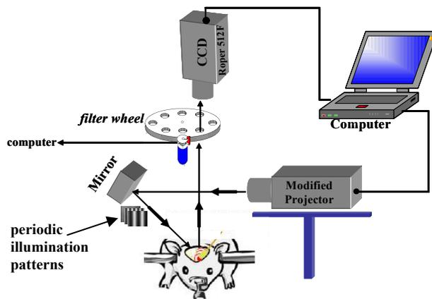
Figure. 1: Schematic of the optical configuration.
