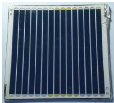
Fig.4. A 10cm-by-10cm sub-module of black-dye-sensitized solar cell and its solar cell performance
