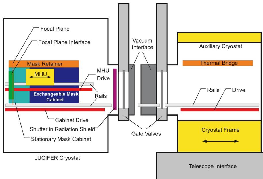
Figure 1: Schematic overview of the MOS system components; see text for details
