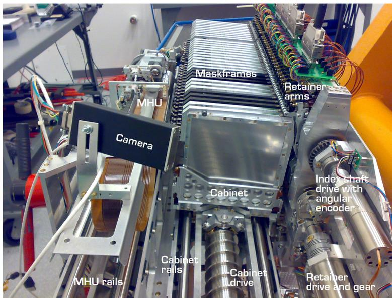
Figure 3: View as seen from the LUCIFER gate valve, the cabinet drive is visible in the front. On the right the motors for the index shaft and drive shaft of the retainer are visible.
