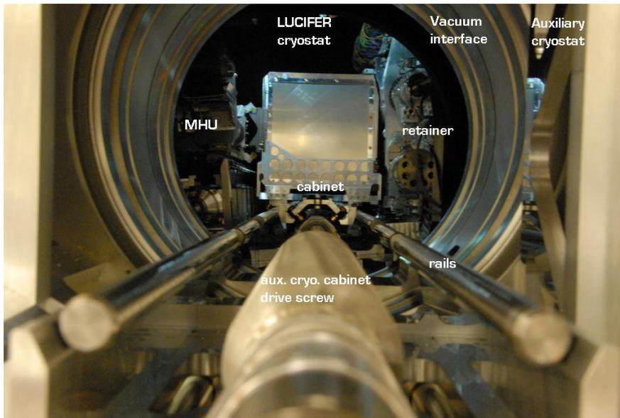
Figure 10: View along the cabinet drive from the auxiliary cryostat towards the Lucifer cryostat. During transfer the cabinet is handed over from the LUCIFER cabinet drive to the Auxiliary Cryostat Cabinet drive in a synchronous motion of the two screws.
