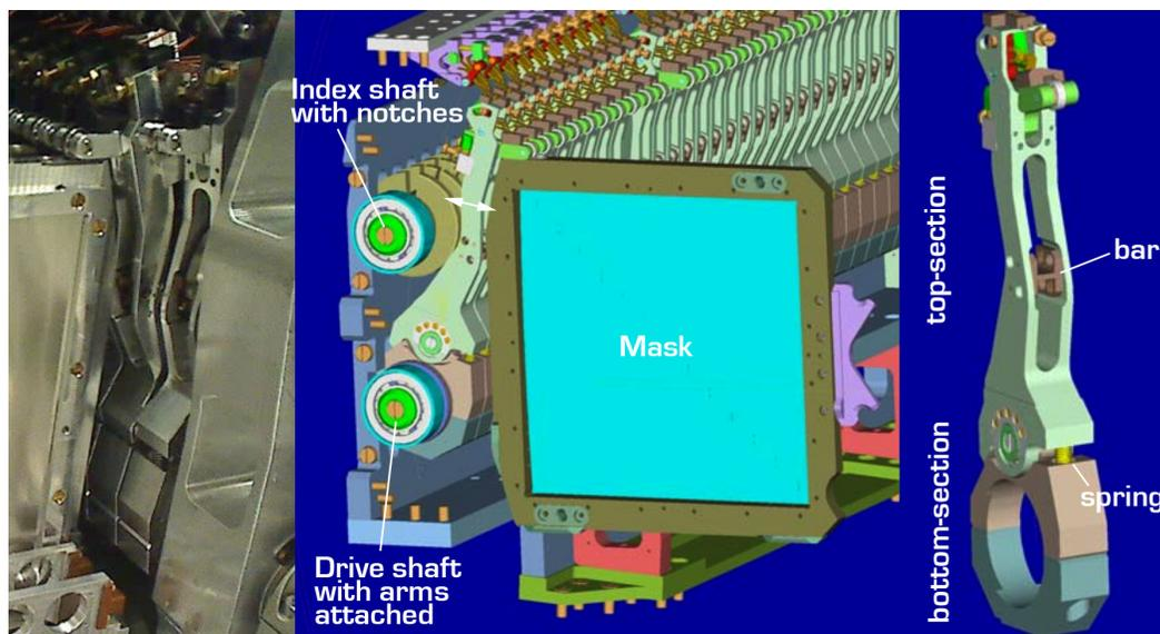
Figure 7: Left: Retainer arms in locked and unlocked position. Note the compressed and expanded springs in the bottom section. Middle: CAD overview of the retainer with drive and index shaft. Right: a single retainer arm
