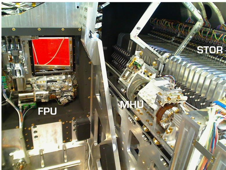
Figure 8: Arrangement of the MOS components inside the LUCIFER cryostat. In the image the MHU is taking a mask out of the cabinet for transport to the FPU. When fully integrated the space left to the MHU is occupied by the folding mirrors and collimator optics.
