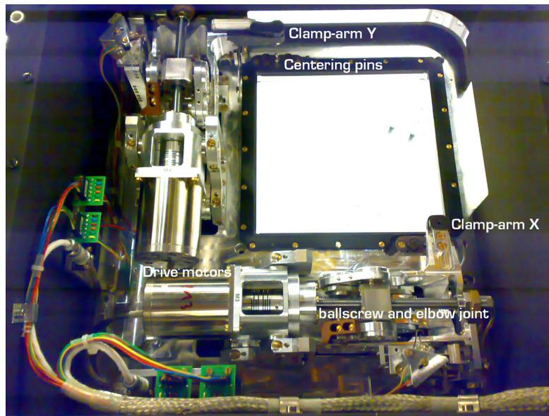
Figure 4: The Focal Plane Unit inside the cryostat. The black frame defines the FOV when no mask is present.
