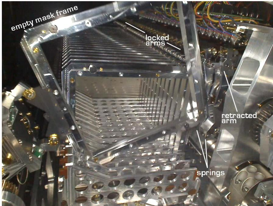
Figure 11: The MHU is taking an empty test mask frame out of the cabinet. On the right: The corresponding arm of the retainer is retracted, all others stay locked. Grabber and mask frame handle can be seen on the left.
