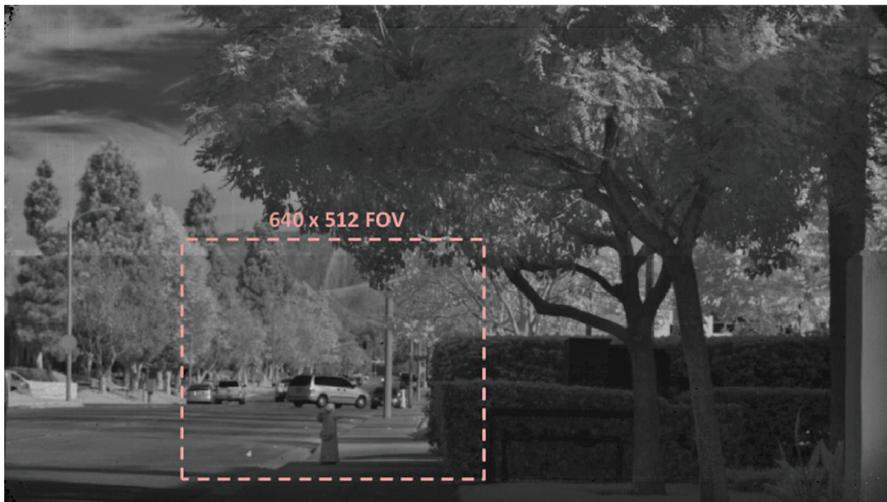
Fig. 13. Daytime imagery taken in integrate while read (IWR) mode from a 1920×1080, 15  $\mu\text{m}$  pixel pitch, low noise InGaAs SWIR sensor. The field of view of a 640×512, 15  $\mu\text{m}$  sensor is shown by the dashed box outline.
