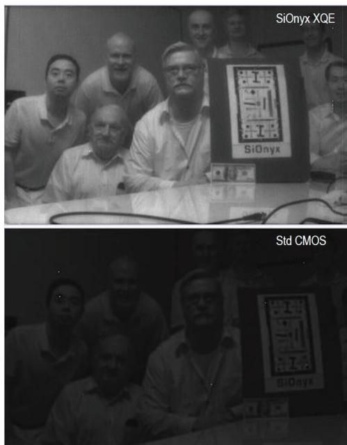
Fig. 56 Images collected in a completely dark room. The only illumination is from a 940 nm LED. The upper image is the XQE sensor and the lower is a standard CMOS sensor. Both sensors have  $380 \times 240$  resolution and  $11.2 \mu\text{m}$  pixels. The integration time for both is 16 msec.
