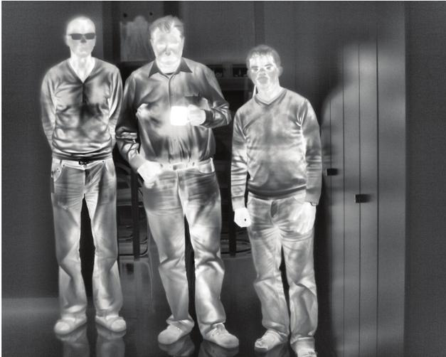
Fig. 25 Image taken with an LWIR HgCdTe FPA having a 1280 × 1024 format and 15 μm pixels.
