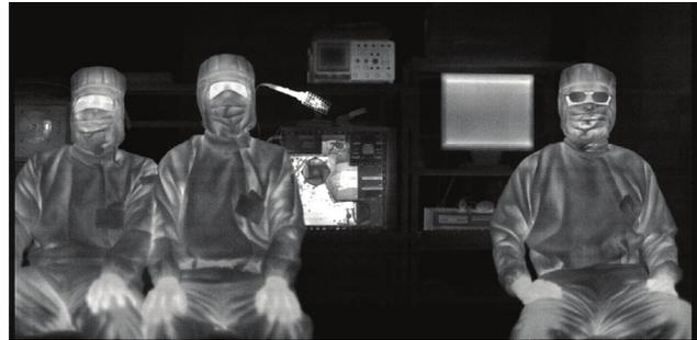
Fig. 44 Image taken with a 2000  $\times$  1000 uncooled array fabricated with SOI technology. NE $\Delta$ T for this 15  $\mu\text{m}$  pixel array was 65 mK.
