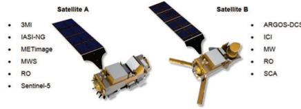
Fig. 2 MetOp-SG, the two-satellite space segment
