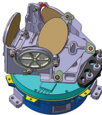
Fig. 3 METImage Derotator Assembly (including mechanism, courtesy of Airbus Defence & Space)
