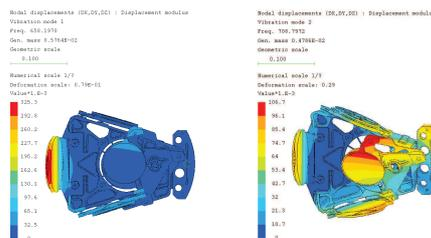
Fig. 5 F.E.M. analysis results (First two modes at 658Hz and 709Hz)
