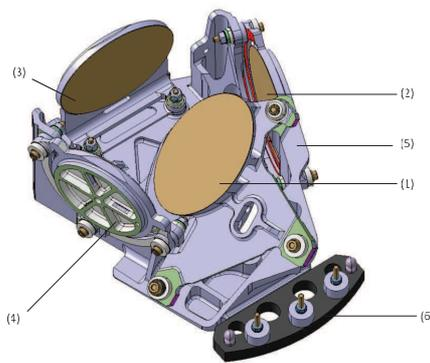
Fig. 4 Derotator Optical Assembly: (5) structural baseplate, (6) counterweight, (1) M1-M5 duplex flat mirror, (2) M2, (3) M3, (4) M4
