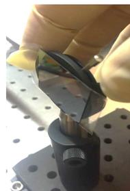
Figure 7: Mounted solid (silicon wafer) sample.
