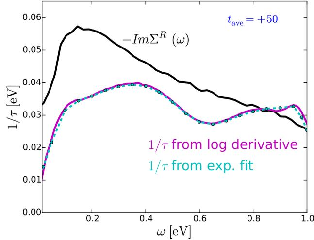
Figure 3. (Color online.) Relaxation rate for different frequency bins at  $t_{ave} = 50 \text{ eV}^{-1}$ . The imaginary part of the retarded equilibrium self-energy is shown for comparison. While there is semiquantitative agreement here, they clearly differ.
