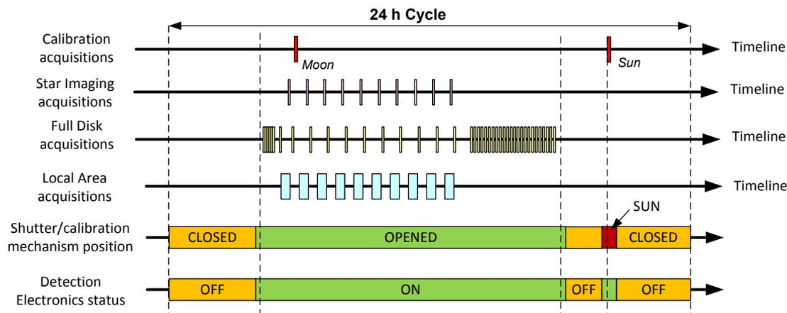
Fig. 6 : Typical example of GOCI-II imaging operation over 24 hours
