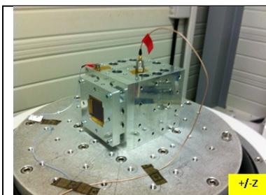
Fig. 22: Detectors during mechanical tests
