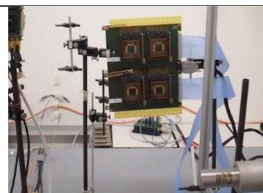
Fig. 23: Detectors during TID irradiation
