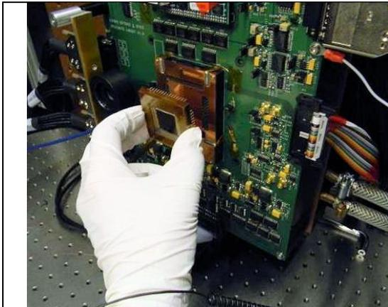
Fig. 18: Detector mounting onto proximity board
