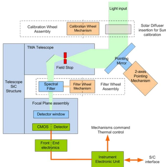
Fig. 3: Functional architecture of the GOCI-II instrument
