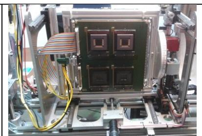
Fig. 24: Detectors during latch-up test (heavy ions)
