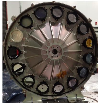
**Fig. 9 : Picture of GOCI-II filter wheel**
