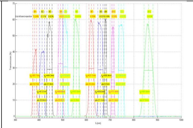
Fig. 19: 12 GOCI-II spectral bands characteristics
