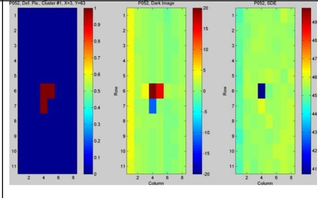
Fig. 21: Cosmetic defects determination for FM selection
