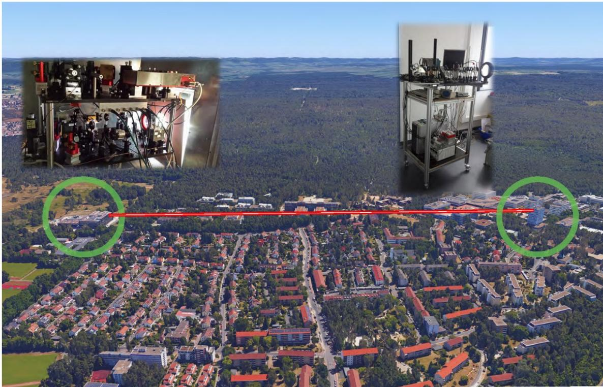
**Fig. 1.** Free space continuous variable quantum link between the new building of the Max Planck Institute for the Science of Light (sender) and the computer science tower of the Friedrich-Alexander University Erlangen (receiver). (Picture of Erlangen: Google)
