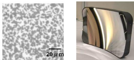
Fig. 12. SiC is porous and needs a polishing layer
