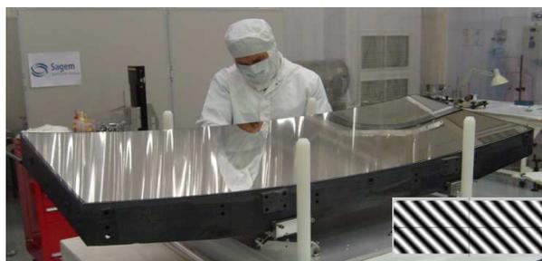
Fig. 13. 150x56 -cm GAIA primary mirror in SiC polished to 9 nm RMS
