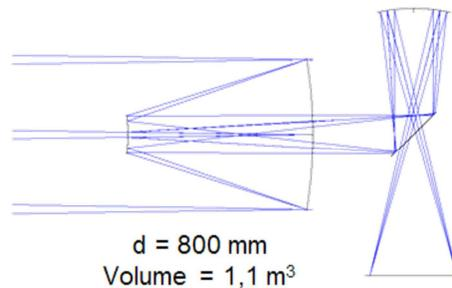
Fig. 3. Compact Pleiades with smart freeforms (same scale as original Pleiades design)
