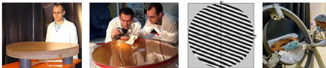
Fig. 11. The extreme OAP as lapped, polished, interferogram and coated
