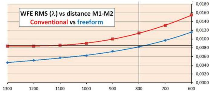
Fig. 2. Performance vs M1-M2 distance and use of smart freeform within the system.
