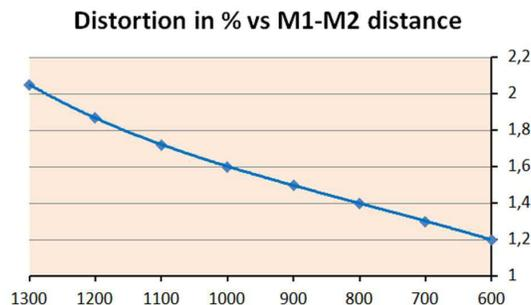
Fig. 4. Distortion reduces with M1-M2 distance
