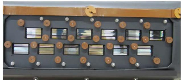
Fig. 5. VNIR FPA PFM, before and after integration of the filters
