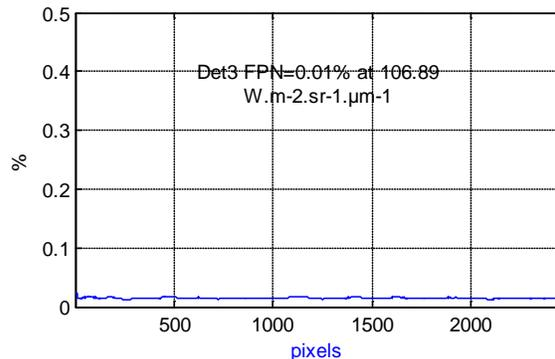
The FPN requirement has been checked on acquisitions performed at Lref over all sections of 100 contiguous pixels.
