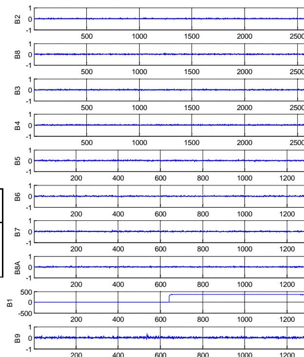
Half line test pattern illuminated on B1 with all the other bands remaining in darkness. Level is plotted for all bands after dark signal subtraction: no visible crosstalk measured.
