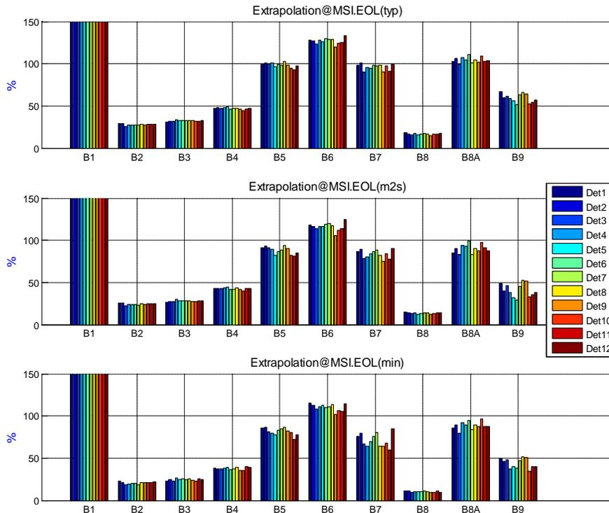
The upper figure provides mean SNR margin for all bands and detectors. The figure in the middle is representative of the performance lower case. The last figure provides the performance of the worst pixel for each detector/band. All pixels are in line with specification with comfortable margin.
