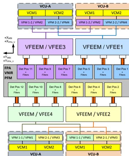
Fig. 4. VNIR FPA detection architecture
