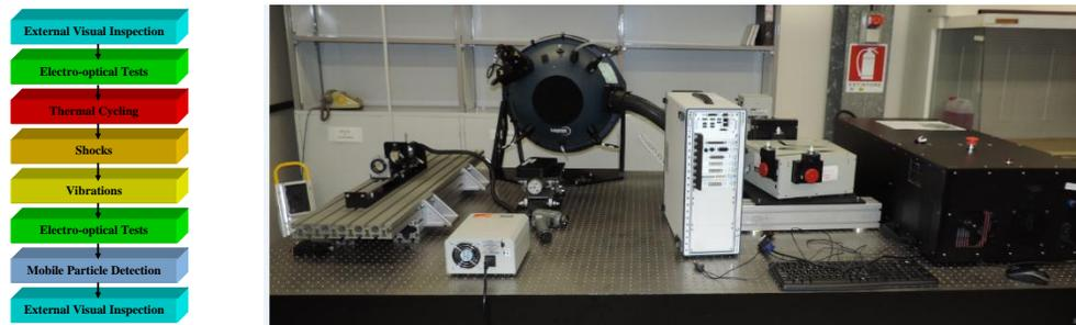
Fig. 13 Characterization sequence (left) and optical setup for EUROCCIS (right).
