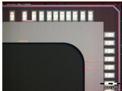
**Fig. 11** Picture of an ARC coated EUROCCIS imager die. The dark region is the AR coated area, the light region is uncoated silicon. The top and right of the picture show the uncoated bond pads.
