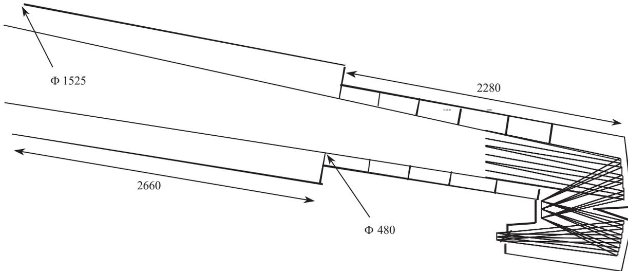
**Figure 5** Baffling concept for a TMA telescope
