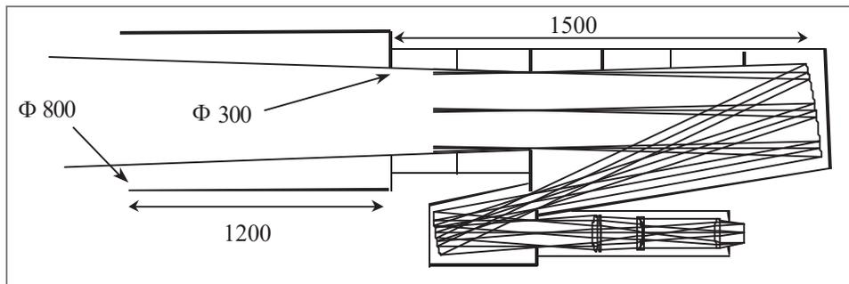
**Figure 6** Baffling concept for the afocal telescope – imaging camera design
