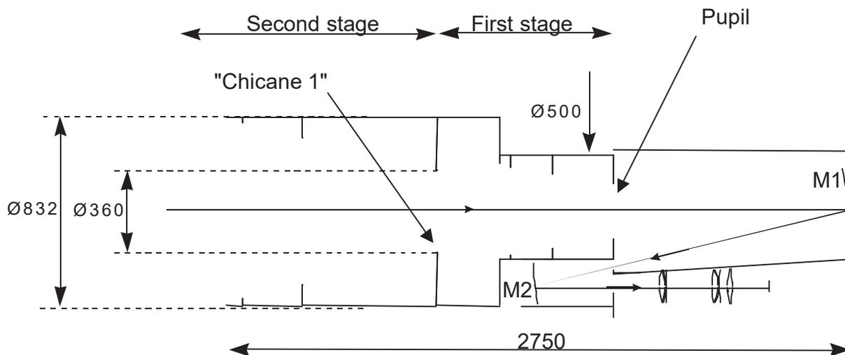
Figure 8 Optimal locations for baffle chicanes
