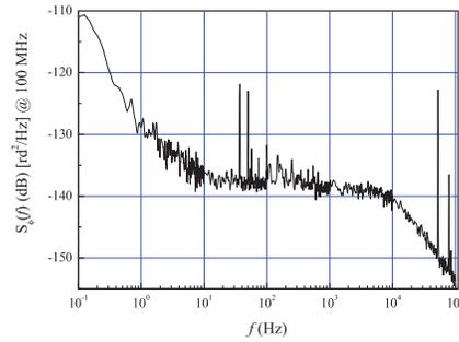
Figure 2. Measured residual phase noise of our transceiver at 1.55  $\mu m$  for a frequency modulation of 100 MHz, a modulation depth of 30% and an optical power of 3 mW.
