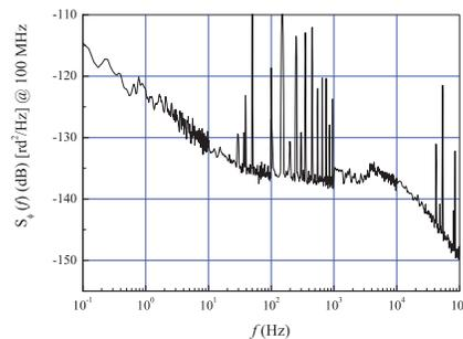
Figure 6. Residual phase noise at 100 MHz of the free-space optical link with compensation.
