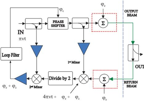
Figure 3. Block diagram of the electronic phase compensation.
