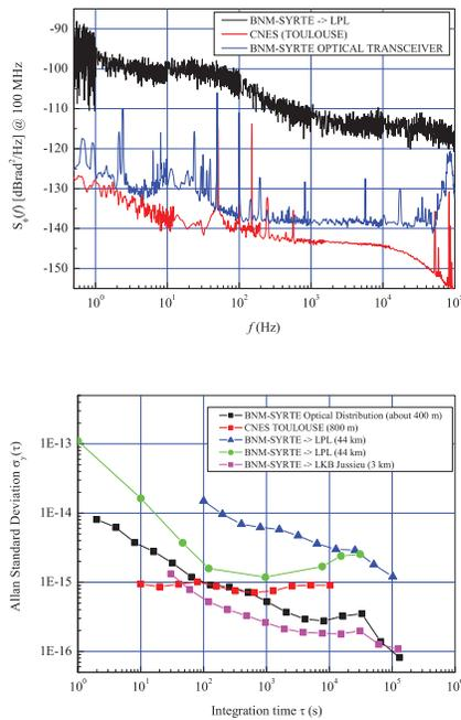
Figure 7. Phase noise and frequency stability measurements realized on the various optical links of BNM-SYRTE.
