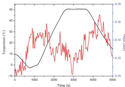
Figure 5. Phase fluctuations at 100 MHz for 50° C temperature variation without compensation and with compensation (1 km fibre spool).
