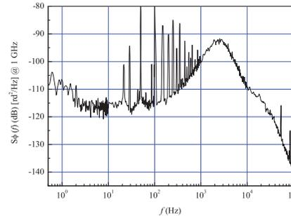
Figure 10. Measured phase noise spectrum of tests with phase compensation breadboard with 2.5 km fibre spool.
