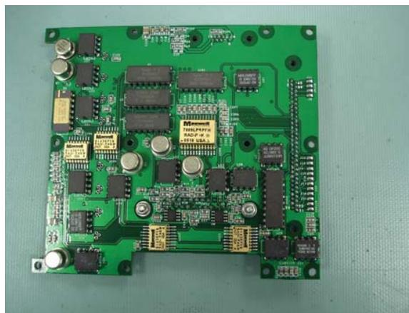
**Fig. 3: Photograph of the low-power flight DAQ (Data Acquisition) PCB.**
