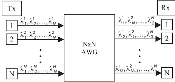
Fig. 1. Basic backplane architecture with NxN AWG.
