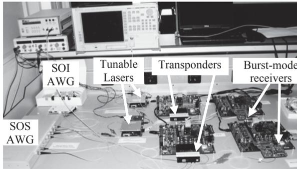
Fig. 2. Photograph of the 4-node demonstrator set-up.
