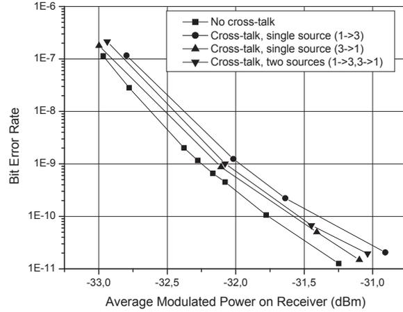
Fig. 4. BER measurements under the presence of coherent cross-talk (CL=13.4db, AWG: SOS)
