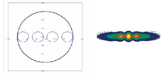
Fig. 5: MTF and associated pupil shape for an incomplete configuration
