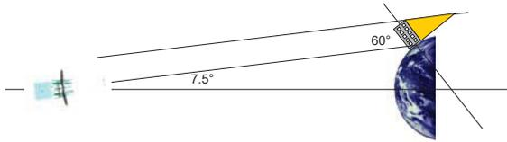
Fig. 2: Masking effect for a resolution of 2 m
