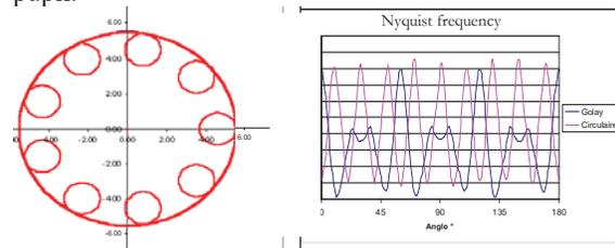
Fig. 9: MTF performances at Nyquist for Golay and circular configuration
