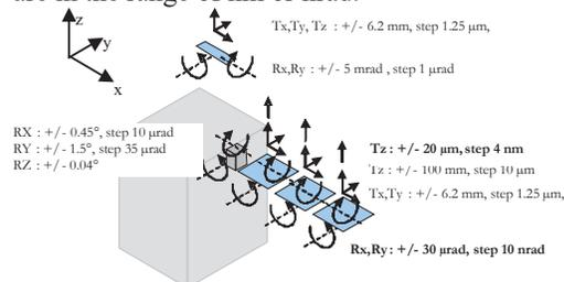
Fig. 11: synthesis of needed mechanisms
