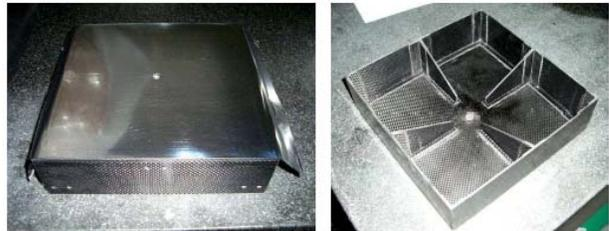
Fig.5. Electrostatic locking breadboard, top and bottom surface. In the top view the Mylar surface is visible.
