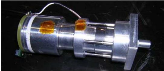
Fig. 2. Active mirror control Actuator.
