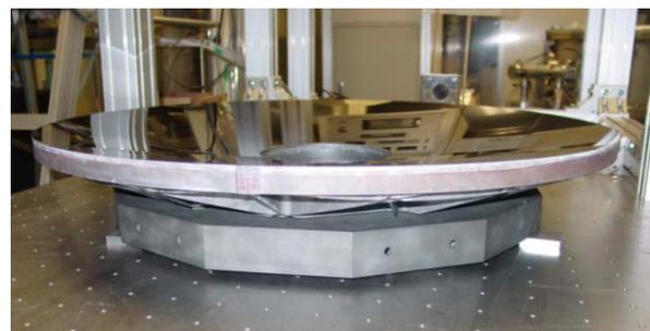
Fig.1 Mirror unit (with supports and optical bench)
