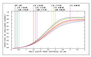
**Fig. 4. EE for the panchromatic filter.** Different lines correspond to different points in the FoV (center, edges, corners). The values are a mean over the wavelength band of the filter.
