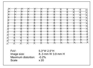
**Fig. 6 Grid distortion for the panchromatic filter.** Note that real chief ray displacements from theoretical values are multiplied by a factor of twenty to make the distortion effects clearly visible.
