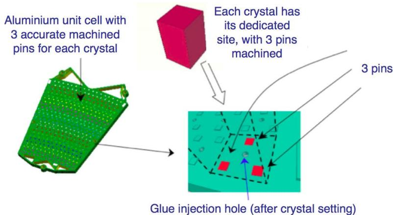
Fig 4 : Method of crystals' fixation proposed by Thales Alenia Space of Cannes for the R&D initiated by the CESR and financed by the CNES. (See text for more details).
