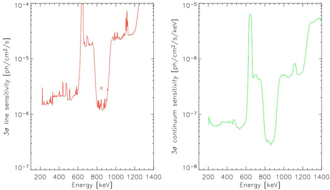
Figure 5 : Narrow line (left panel) and continuum (right panel) sensitivity of GRI telescope in the energy band covered by the Laue lens. These calculations assume 100 ks of exposure time, and an energy bin of  $E/2$  for the continuum sensitivity. On the left panel, the cross shows the sensitivity for the 847 keV broadened line.
