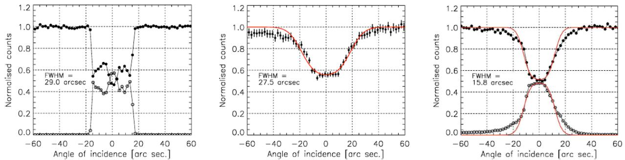
Fig 2 : Left: RC of a 23 mm thick SiGe gradient crystal measured at 300 keV (reflection 111). Center: RC of a 8.6 mm thick Cu crystal (220 reflection) realized at 489 keV. Right: RC of a 2 mm thick Au crystal (reflection 111) realized at 588 keV. Applying the transmission coefficient due to the absorption through the crystal, the achieved reflectivities are respectively: 0.26, 0.24 and 0.31. All these measurements have been performed at ESRF (Grenoble France) on beamline ID15A.
