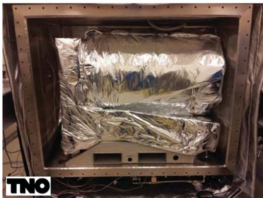
Fig. 5. Realized Thermal Vacuum Chamber setup.
