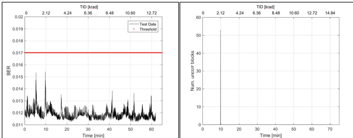
Figure 7. AC100M gamma radiation test campaign results; (left) Bit error rate recorded over time for testing below TID level of ~13.7 krad; BER was below 0.017 threshold. (right) AC100M receiver number of uncorrected blocks recorded over time. One occurrence of a number of uncorrected blocks (53) greater than zero.
