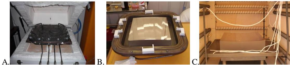
**Fig. 2.** (A) Muffle used for the direct slumping; (B) fused silica mould in the muffle; (C) mould and foil into the furnace used for the indirect slumping tests.
