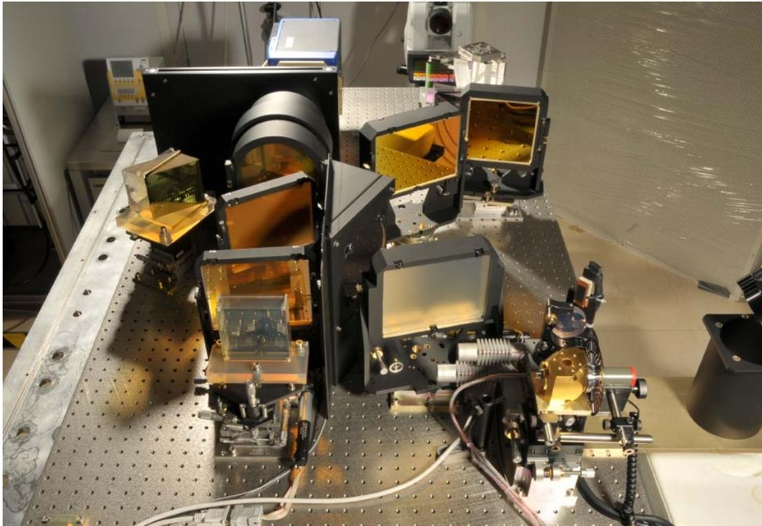
**Fig. 3.** Picture of the main bench of MOPI. The interferometric core (staircase mirrors, beam splitter and modulation plate) is on the foreground, on the left. The commercial detector used on the beginning of the measurements is on the background. The right part of the bench consists in the calibration part. The cold box was not implemented at the time the picture was taken.
