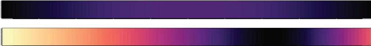
Figure 5. Wavefront error map: Center slit (top) with range 80.4 nm to 134 nm. Outer slits (lower) with WFE range 45 nm to 284 nm. In the outer slits, the WFE is highest at the innermost ends of the slits (light colour); in the centre slit the WFE is highest in the centre of the slit.
