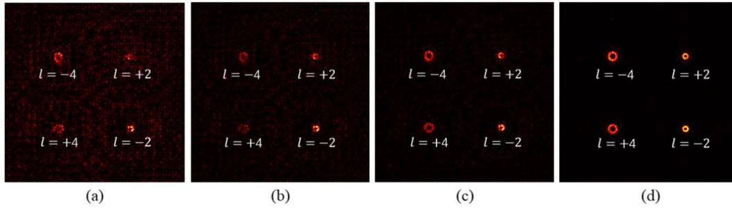
Figure 1. Schematic diagram of the optimization effect based on the PSO algorithm. The optimization results of OV array intensity distribution for 60 particles from (a) to (d) for 50, 100, 500 and 1000 iterations respectively. It can be seen that the noise of the OV array image is reduced, the signal is enhanced, and the intensity distribution of OV tends to be uniform
