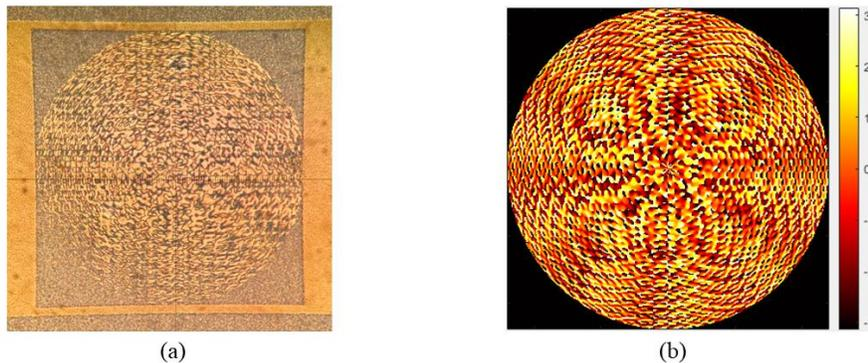
Figure 2. (a) Picture of LCD under polarization microscope, the working area of the LCD is a circle with a diameter of 2mm, (b) LCD phase distribution calculated based on vector diffraction theory.
