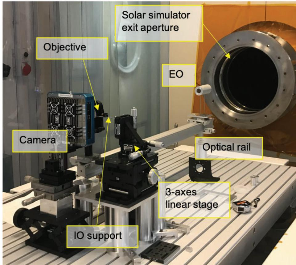
Figure 5: Picture of the SailCor prototype in front of the solar simulator source at the OPSys facility in Torino.
