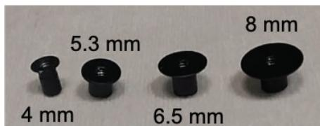
Figure 11: The full series of manufactured IOs. Diameters are specified by labels.
