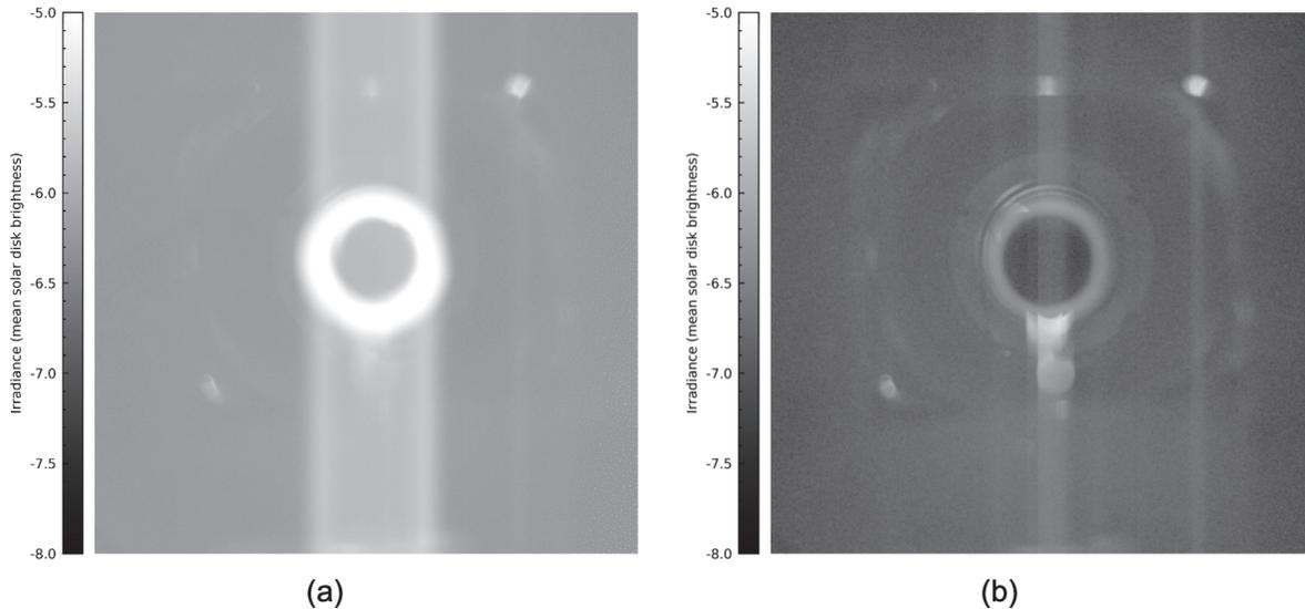
Figure 15: Stray light images with the sand blasted cone EO. Units are mean solar disk brightness irradiance in log scale. (a) Without EA. (b) With EA.
