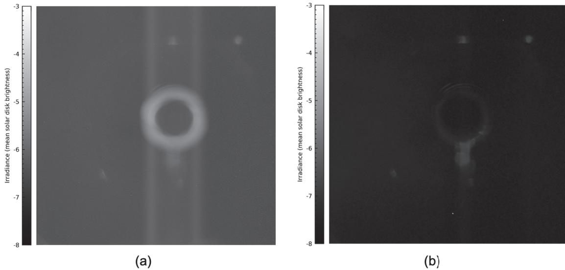
Figure 14: Stray light images with the polished cone EO. Units are mean solar disk brightness irradiance in log scale. (a) Without EA. (b) With EA.
