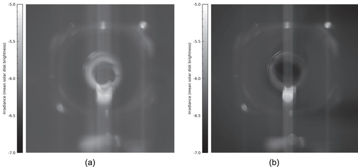
Figure 13: Stray light images with the triple disk EO. Units are mean solar disk brightness irradiance in log scale. (a) Without EA. (b) With EA.
