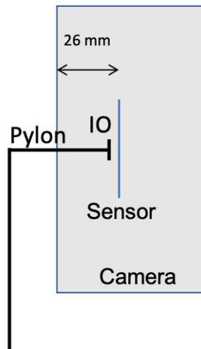
Figure 9: A sketch of the IO positioning principle.
