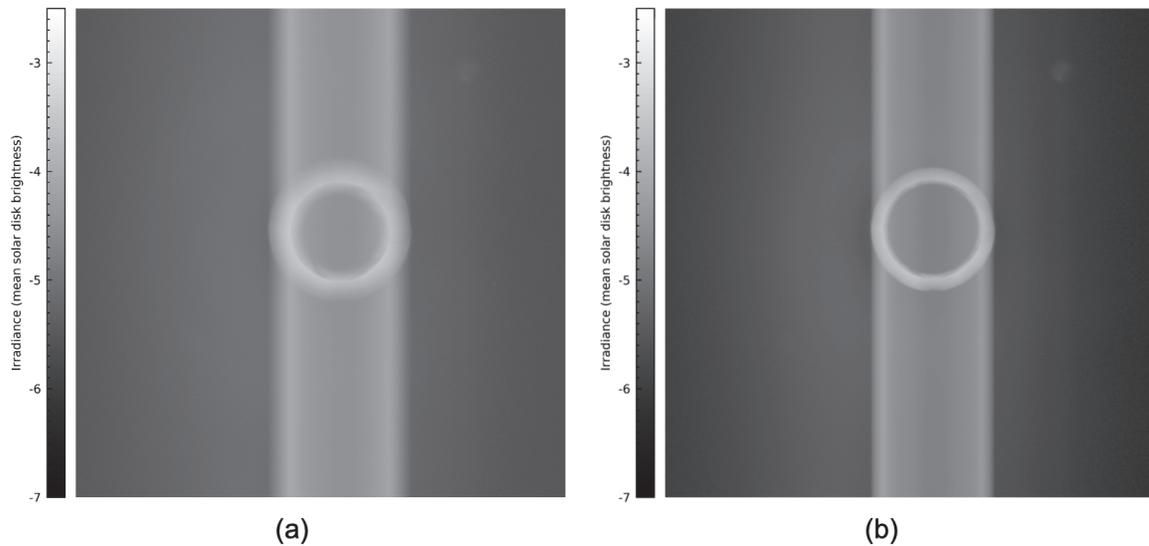
Figure 12: Stray light images with the simple disk EO. Units are mean solar disk brightness irradiance in log scale. (a) Without EA. (b) With EA.
