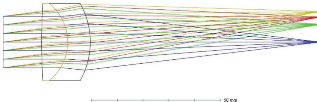
Figure 7: Ray tracing on the objective lens.
