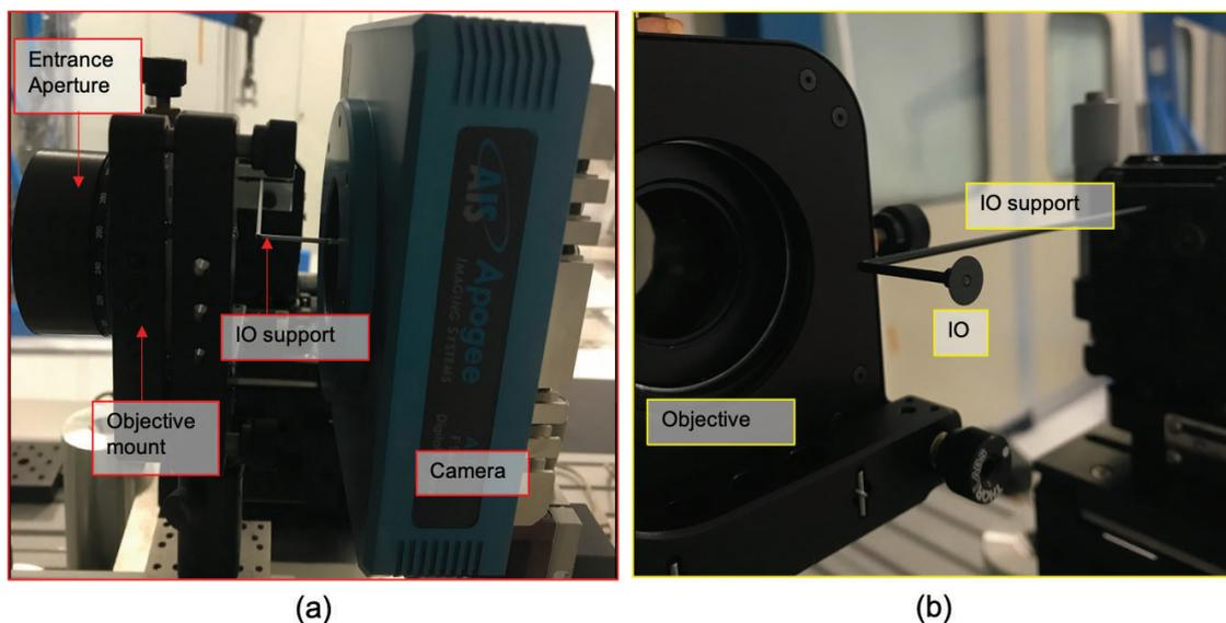
Figure 10: (a) Objective assembly with the entrance aperture, IO support and camera. (b) Zoom on the IO by removing the camera.
