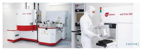
Figure 6: Ion Beam Figuring machine (left) including a fully automated wafer cassette loader (right), as recently installed at cosine.
