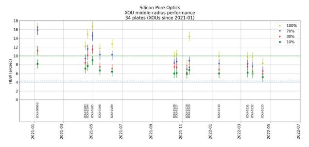
achieve a HEW of about 7", as shown in figure 5 (independent measurements taken at the PANTER facility). For more details on these measurements see [23].
