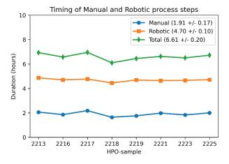
Figure 3: Pilot-production run of middle radius stacks using one stacking robot, showing manual, automated and total times for each of the 8 stacks (identified by their HPO number).
