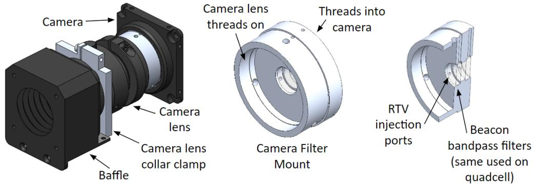
Figure 10: CLICK-B/C beacon camera assembly. The baffle is also coated in a black coating to reduce stray light reflections.
