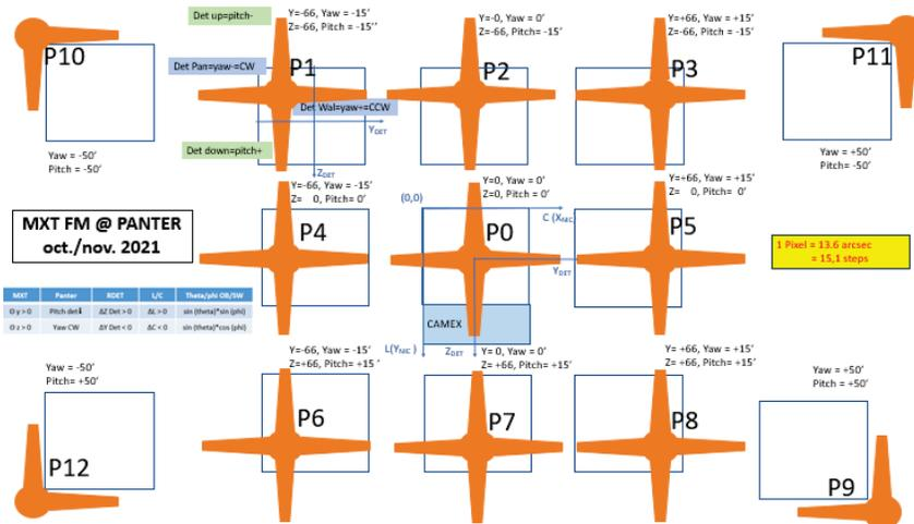
Figure 8 Measurement strategy showing the positions chosen for the location of the PSF on the detector with the corresponding pitch and yaw angles to which the telescope has to be oriented to.
