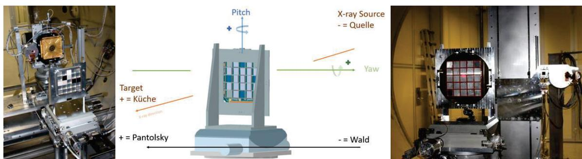
Figure 1 SVOM-MXT-MOP optics in the PANTER vacuum chamber, view from the source toward the detector: (left) the Bread-Board (BB) and (right) the Qualification Model (QM) models are shown. (center) shows the coordinate system used in PANTER during the optics measurement campaigns. During the BB measurements, the Position Sensitive Proportional Counter (PSPC), a ROSAT flight spare, was also used for measurements together with the TRoPIC pnCCD camera.
