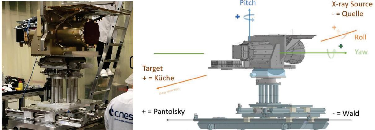
Figure 5 (left) Photograph showing the SVOM-MXT-PM model telescope being mounted onto the PANTER manipulators in the grey area. (right) shows the coordinate system used during the telescope tests.
