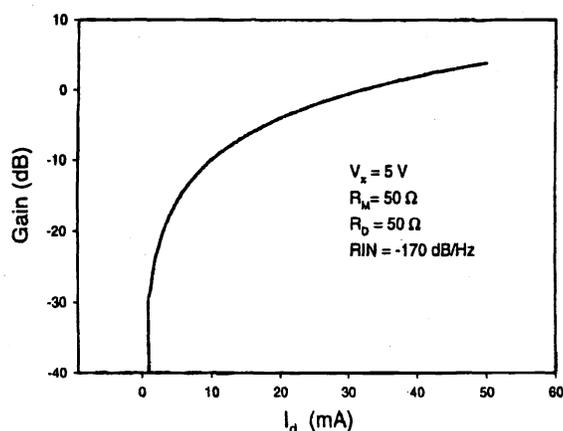
Figure 3: Link Gains vs. Photodetector Current
