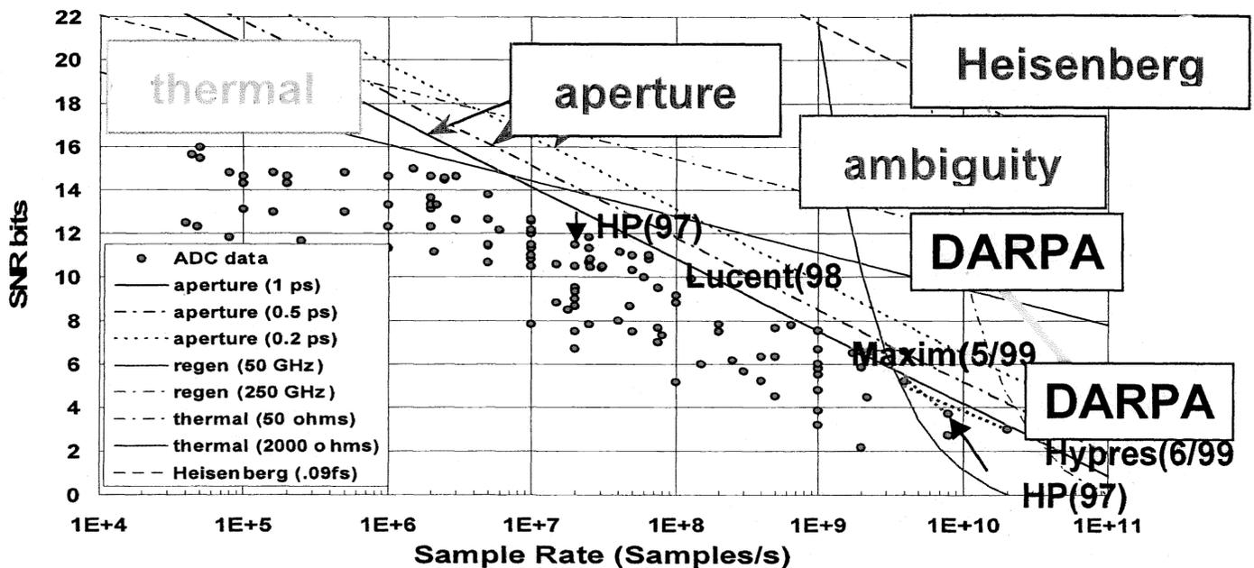
Figure 4: Electronic ADC Evolution / "The Walden Wall"
