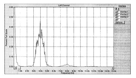
Fig. 2. Doppler frequency shift power spectrum obtained with rotating frozen glass disk.
