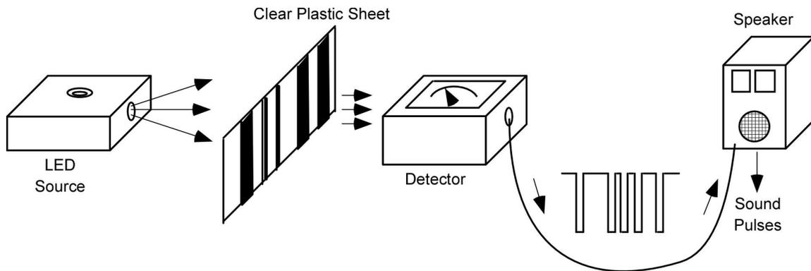
Figure 5. Barcode reader kit configuration.
