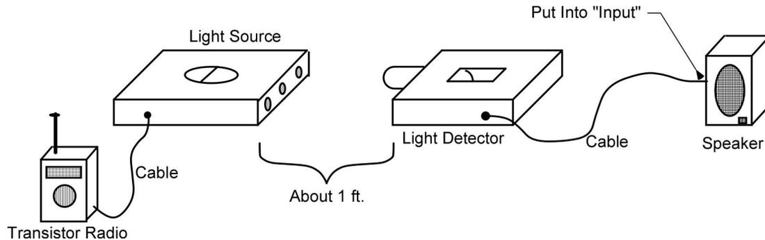
Figure 6. Communication by Light kit setup.
