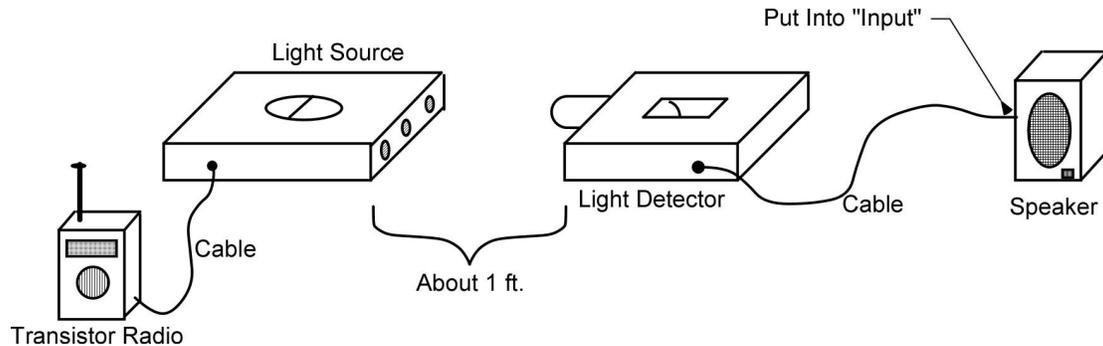
Figure 6. Communication by Light kit setup.
