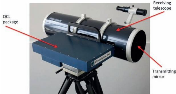
Figure 10. Photograph of standoff explosives sensor on a tripod
