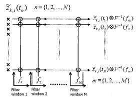
**Fig. 1** Schematic of the sliding-window filtering technique. The sliding-window filtering bank is used to measure the components of each interference signal that change at a rate corresponding to the passband of the filters.
