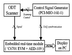
Fig. 2 Schematic of the DSP-based ODT system.
