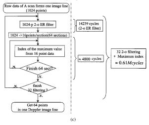
**Fig. 6** Code structures of three processing modes: (a) Structural imaging, (b) weighted-centroid flow imaging, (c) sliding-window filtering flow imaging.
