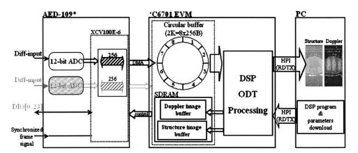
**Fig. 5** Data flow in the DSP-ODT system: hardware perspective. An eight-frame circular buffer in the 'C6701 DSP continuously receives 12-bit data from the AED-109 analog daughterboard; the DSP module simultaneously processes data in each frame; a PC loads the image data right after processing through the host-port interface (HPI).
