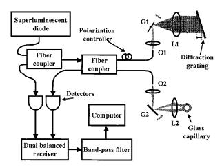
**Fig. 3** The ODT scanner, which is a typical balanced setup with both axial and lateral scanning, performed by a galvanometer. O1, O2, microscope objectives; G1, G2, galvanometers; L1, L2, achromatic lenses.
