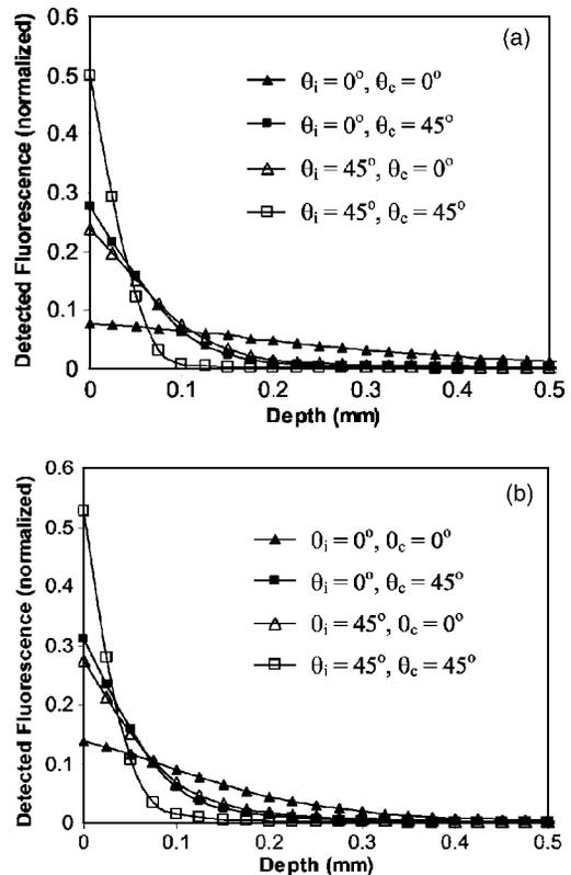
**Fig. 2** Depth-resolved graphs of the effect of illumination and collection angle on relative sensitivity for overlapping spot designs. Graphs present data for (a) low and (b) high attenuation cases. Label for each curve indicates type of illumination and collection geometry, respectively. Data have been normalized to total detected signal.
