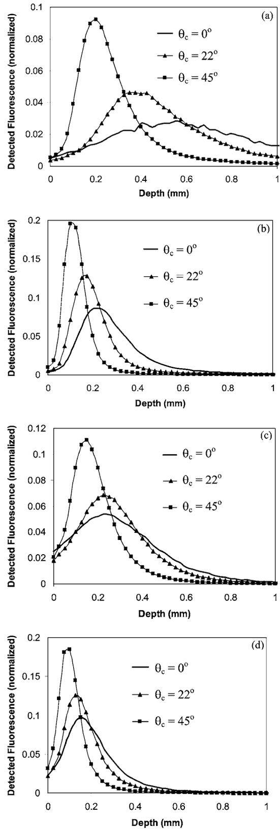
**Fig. 4** Effect of illumination and collection angle for nonoverlapping geometries where  $L=0.1$  mm. The four graphs represent two optical property sets and two illumination geometries: (a) low attenuation,  $\theta_i=0$  deg; (b) low attenuation,  $\theta_i=45$  deg; (c) high attenuation,  $\theta_i=0$  deg; and (d) high attenuation,  $\theta_i=45$  deg. For each graph, three collection angles are presented as specified.
