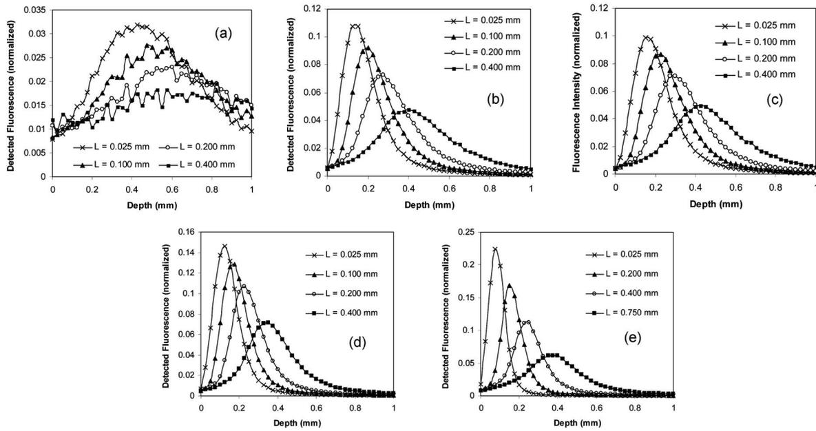
**Fig. 5** Effect of spot separation distance ( $L$ ) for the low attenuation case. The five graphs represent different illumination-collection geometries: (a)  $\theta_i=0$  deg,  $\theta_c=0$  deg; (b)  $\theta_i=0$  deg,  $\theta_c=45$  deg; (c)  $\theta_i=45$  deg,  $\theta_c=0$  deg; (d)  $\theta_i=45$  deg,  $\theta_c=22$  deg; and (e)  $\theta_i=45$  deg,  $\theta_c=45$  deg. Note that a different set of separation distances were used in (e).
