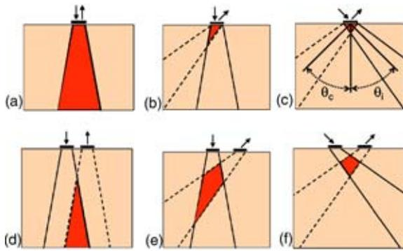
**Fig. 1** Illustration of illumination (solid lines) and collection (dashed lines) cones for normal- and oblique-incidence geometries. Darkened areas indicate the regions of overlap, and thus maximum sensitivity. Diagram in (c) indicates how illumination ( $\theta_i$ ) and collection ( $\theta_c$ ) angles were defined.
