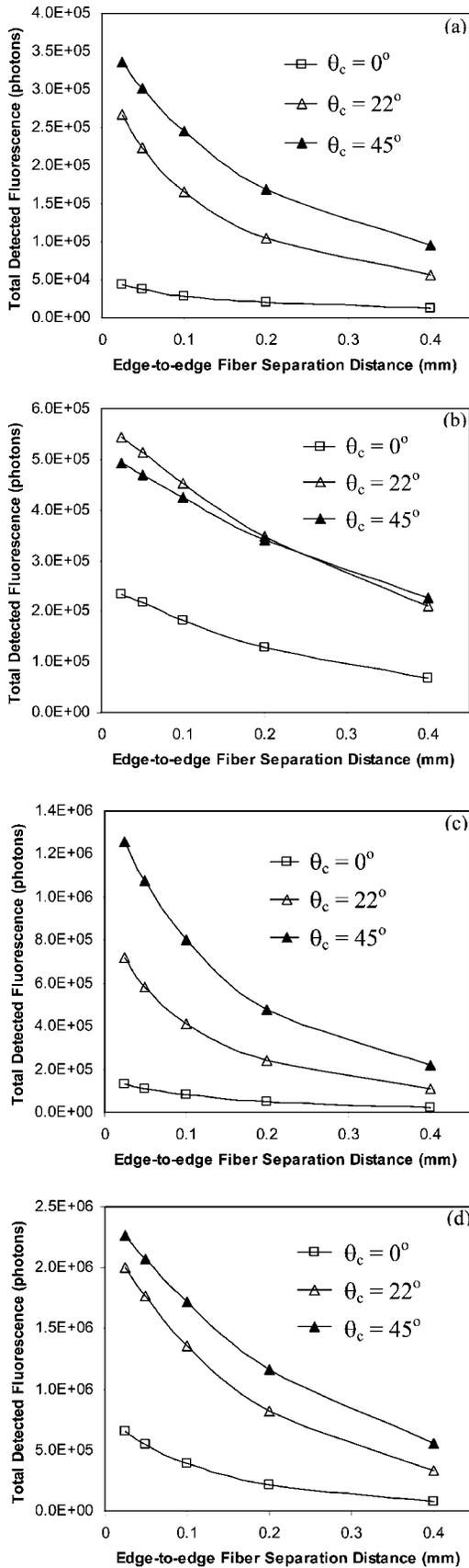
**Fig. 7** Detected signal intensity as a function of probe design for (a) low attenuation  $\theta_i=0^\circ$ , (b) low attenuation,  $\theta_i=45^\circ$ , (c) high attenuation,  $\theta_i=0^\circ$ , and (d) high attenuation  $\theta_i=45^\circ$ .
