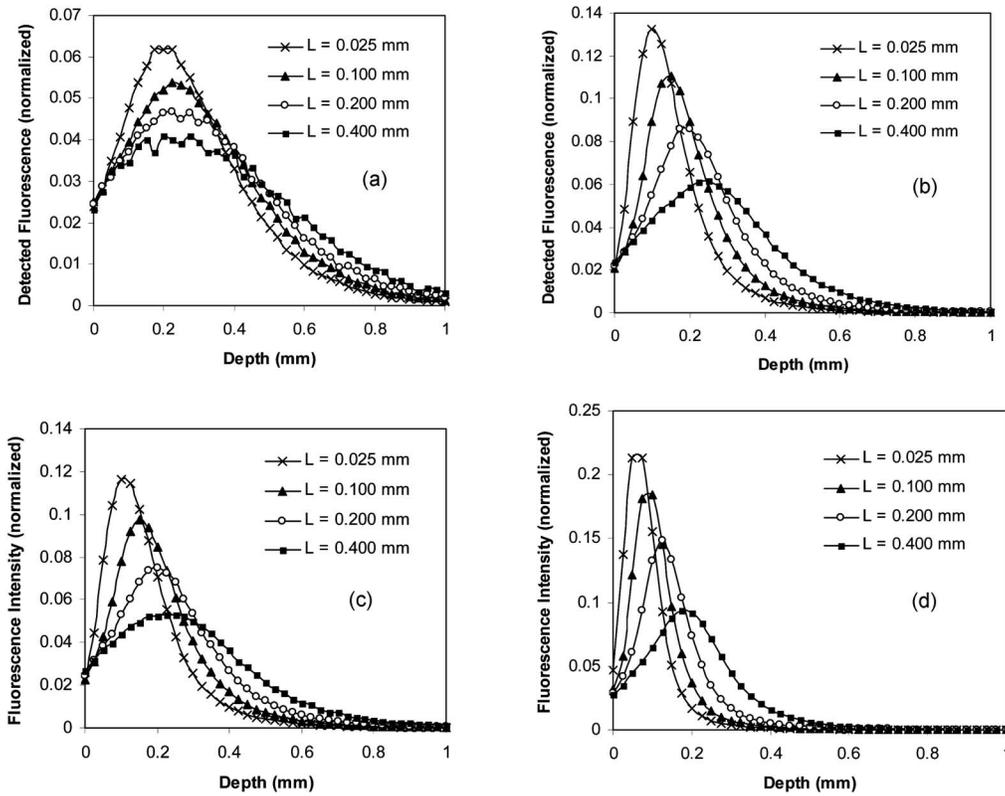
**Fig. 6** Effect of illumination-collection spot separation distance ( $L$ ) for the high attenuation case. The four graphs represent four cases: (a)  $\theta_i=0$  deg and  $\theta_c=0$  deg; (b)  $\theta_i=0$  deg and  $\theta_c=45$  deg; (c)  $\theta_i=45$  deg and  $\theta_c=0$  deg; and (d)  $\theta_i=45$  deg and  $\theta_c=45$  deg.
