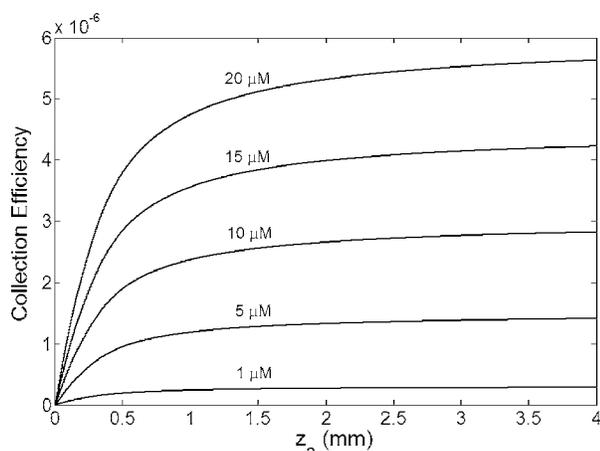
**Fig. 3** Theoretical fluorescence collection efficiency curves for a single fiber probe immersed in rhodamine:6G (Rh:6G), using molar concentrations in the range 1 to 20  $\mu\text{M}$ . The NA and core diameter of the fiber were 0.22 and 105  $\mu\text{m}$ , respectively; the refractive index of the sampling volume was 1.34; and the quantum efficiency ( $\eta$ ) was set to unity.
