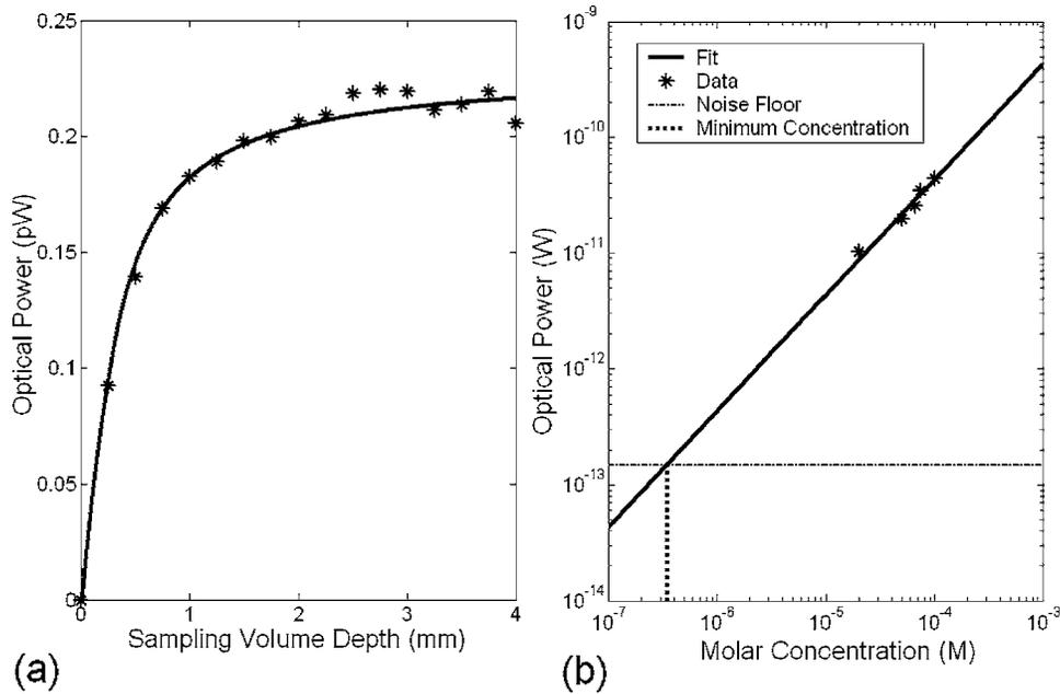
**Fig. 5** (a) Fluorescence signal power versus sampling volume depth: experiment ( $\hat{\cdot}$ ), theoretical fit (solid line). Concentration of Rh:6G is  $1 \mu\text{M}$ . (b) Plot of the fluorescence signal power versus the fluorophore (Rh:6G) concentration: experiment ( $\hat{\cdot}$ ), linear fitting (solid line), noise floor (dashed-dotted line).
