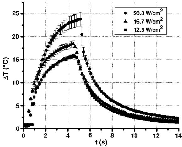
Fig. 3 Mean temperature rise measured on cornea external surface, for a 5-s single spot irradiation and three different laser power densities.
