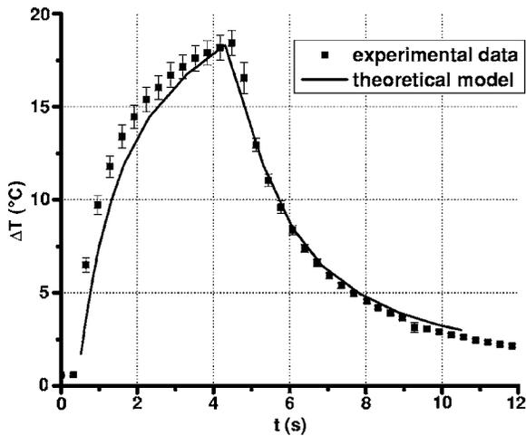
Fig. 4 Temperature rise of a laser-welded cornea external surface, calculated within the mathematical model (continuous line). Mean value experimental data are shown (symbols), as a reference. Calculations and data refer to a 5-s treatment time with 16.7 W/cm<sup>2</sup> laser power density.
