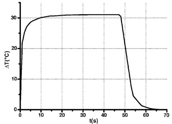
Fig. 6 Calculated temperature rise for a 50 s irradiation time of an ICG-stained cornea at a power density of 12.5 W/cm<sup>2</sup>. Data refer to the maximum temperature inside the corneal tissue.
