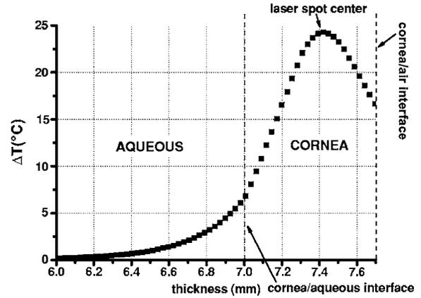
Fig. 5 Temperature rise distribution along radial distance from the center of the eye toward external ambient air. These calculated data refer to 12.5 W/cm<sup>2</sup> laser power density and 2-s treatment time. The  $\Delta T$  maximum value is inside the cornea, in correspondence with the laser spot center.
