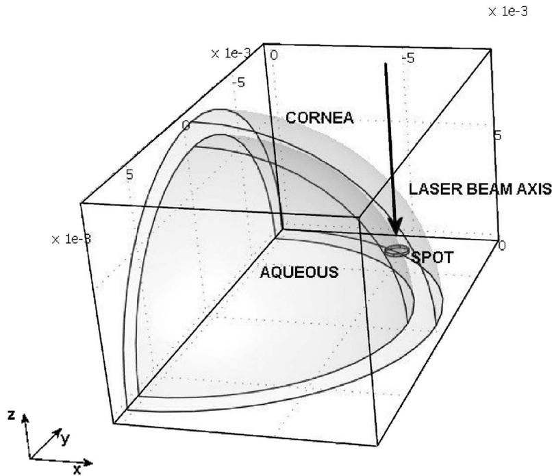
Fig. 2 Eye geometrical model during laser welding of a corneal cut.
