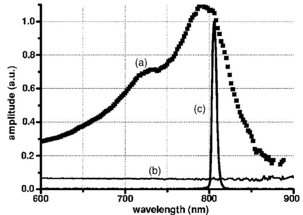
**Fig. 1** Absorption curve of an ICG-stained porcine cornea (a) and of a native cornea (b). Diode laser peak wavelength is also shown (c).
