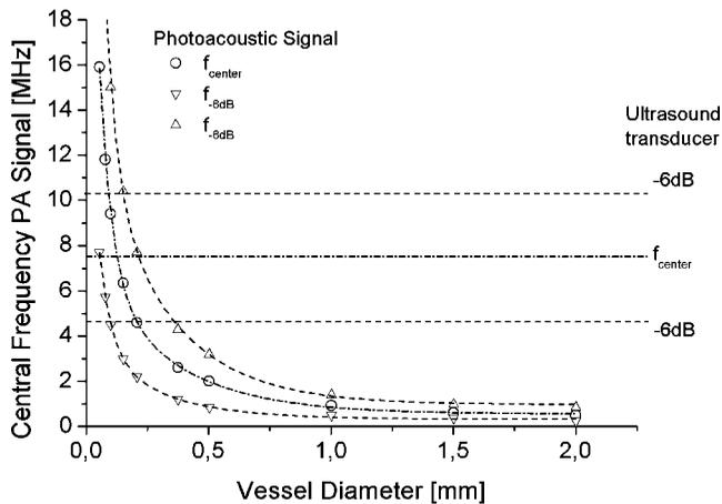
**Fig. 3** Central frequency and  $-6$ -dB bandwidth of the photoacoustic signal as a function of vessel diameter. The central frequency and  $-6$ -dB bandwidth of the 7.5-MHz transducer are plotted as well (horizontal dashed lines).
