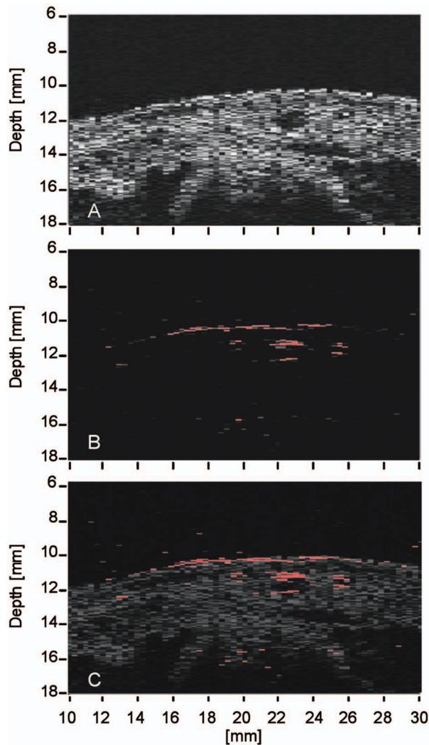
**Fig. 2** Images of the dorsal side of the left hand of a human volunteer: (a) ultrasound image, (b) photoacoustic image, (c) combined image. The acquisition time for the images was 128 msec (8 frames/sec).
