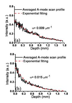
**Fig. 9** A-mode scan profiles (solid curves), averaged over a lateral scan range of 100  $\mu$ m, of the (a) ES-SCC and (b) WD-SCC cases. The exponential decay fitting curves (dashed curves) are also shown. The decay constant,  $\alpha$ , values are indicated.
