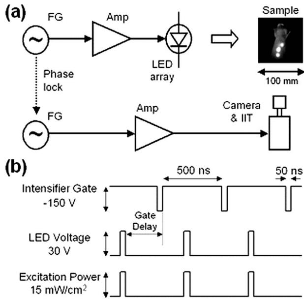
**Fig. 1** (a) Schematic diagram of wide-field time-gated imaging system. Phase-locked function generators (FG, Agilent 33250) are amplified (ENI 350L RF power amp) to provide the drive voltage for the light source (Luxeon ND93LXHL LED array) excitation and image intensifier tube (IIT, Hamamatsu V7090U-71-G130RG/NG) photocathode modulation. The IIT phosphor is imaged by a CCD camera (Basler A312f) operating at 8 fps. (b) Timing diagram for excitation and detection gating.
