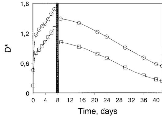
**Fig. 12** The temporal dependence of  $D^*$  for *in vivo* human skin with developing erythema: (○)  $\lambda = 460$  nm; and (□)  $\lambda = 500$  nm.
