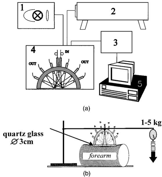
**Fig. 1** (a) Experimental setup: (1) xenon arc lamp; (2) N<sub>2</sub> gas laser; (3) monochromator; (4) fiber-optical probe; and (5) PC. (b) Special device for external mechanical compression of the human skin *in vivo*.
