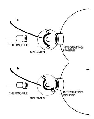
Fig. 2 Cartilage reshaping jig. (a) The cartilage specimen is held in compression between two aluminum rods 2.5 cm apart mounted on a rotational stage. In reshaping experiments only I(t) and S<sub>c</sub>(t) are monitored. I(t) is monitored on the lock-in amplifier display, and when d(I(t))/dt≈0 laser irradiation is stopped. (b) Following laser irradiation, the stage is then rotated to a new position so that nonirradiated tissue can be brought into the laser irradiation zone.
