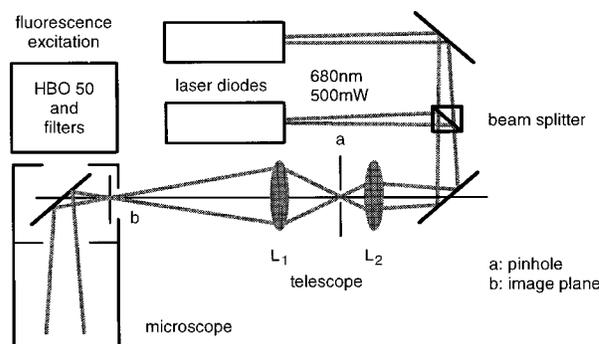
**Fig. 1** Optical setup for laser tweezers using two high power laser diodes (500 mW) together with a fluorescence microscope (sample and objective lens are omitted).
