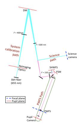
**Fig. 2** Schematic of wavefront sensing bench containing a PWFS and an SHWFS. The green box indicates the elements that are changed for each of the three PWFS.
