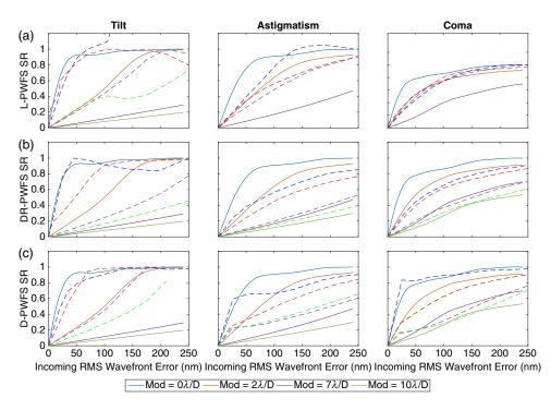
**Fig. 4** Idealized PWFS SR curves (solid) for three Zernike modes with varying modulation along with the experimental data shown by the dashed lines. (a) L-PWFS, (b) DR-PWFS, (c) D-PWFS. The dynamic range refers to the range for which the PWFS is linear.
