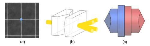
**Fig. 1** Three different PWFSs tested in this work. (a) Lenslet array with a blue dot illustrating where the focal spot should hit the array to form a PWFS. (b) Schematic of a DR-PWFS. (c) The D-PWFS for the LBT, similar to the one used in this work.<sup>7</sup>
