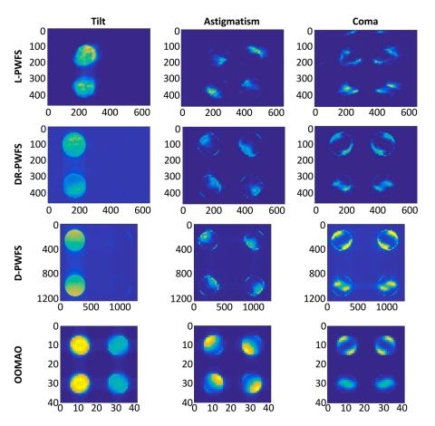
**Fig. 3** PWFS pupils for three Zernike modes with a 100-nm RMS wavefront error and a modulation radius of  $2\lambda/D$ . Note that the D-PWFS pupil was imaged using a different camera than the other L- and DR-PWFS. This is indicated by the *x* and *y* axes, which show the camera pixels.
